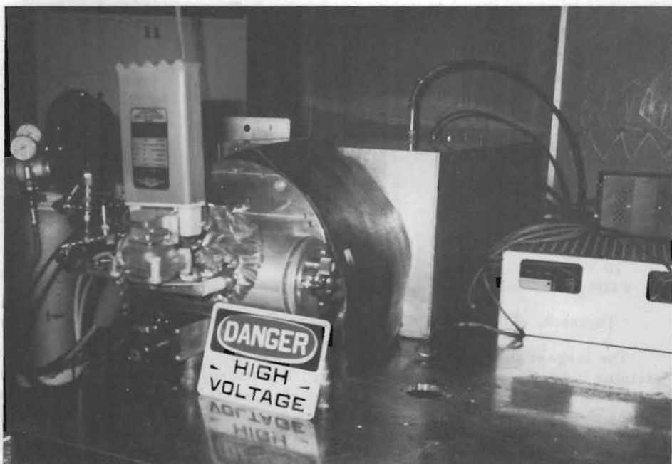
Figure 9. E-Beam Sustained Discharge Laser
